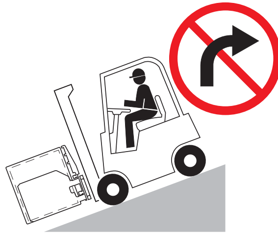
禁止坡上转弯 No turning on ramp
