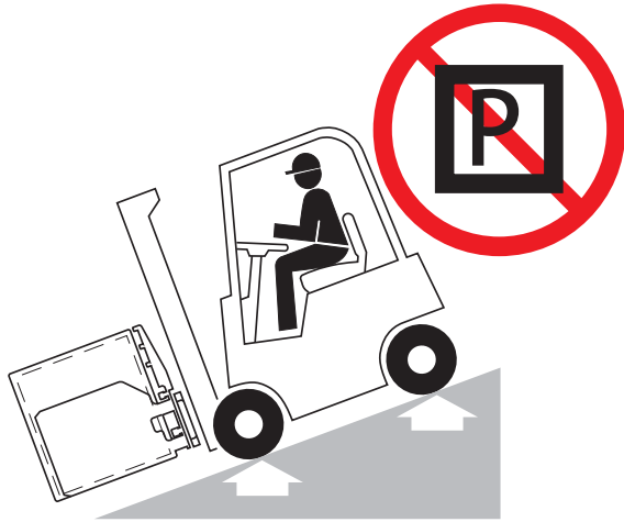
禁止坡上停车 No parking on ramp
